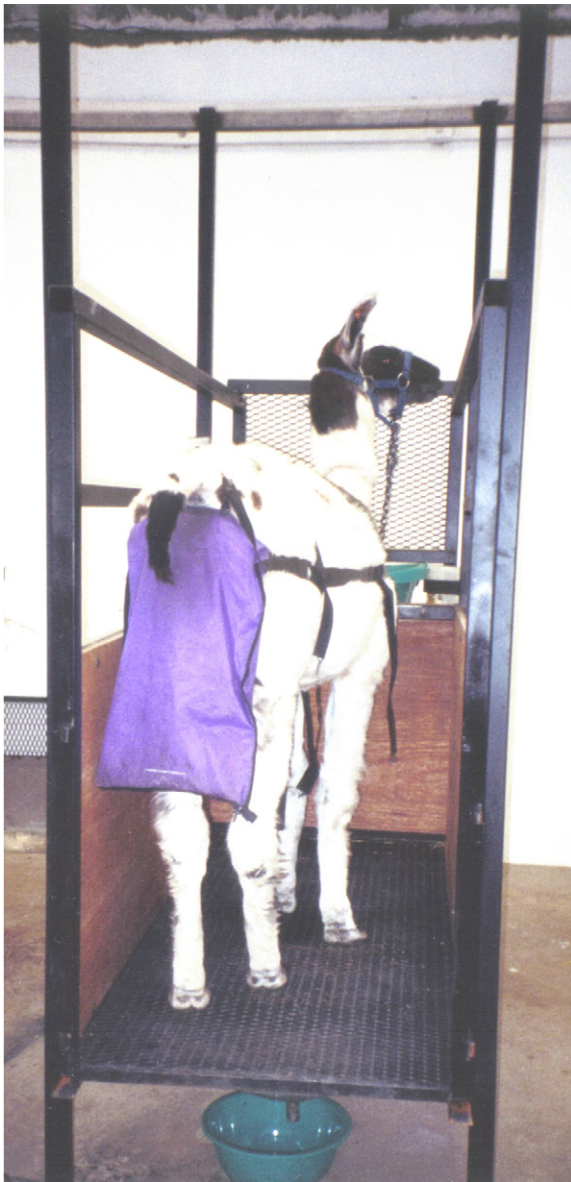
Fig. 1. Llama housed in metabolism crate with fecal collection bag and urine collection tray with attached funnel.
